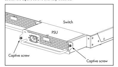
If a unit is already in the bay, slide it out slowly and carefully. Support the unit from underneath as you remove it to prevent it from falling.
